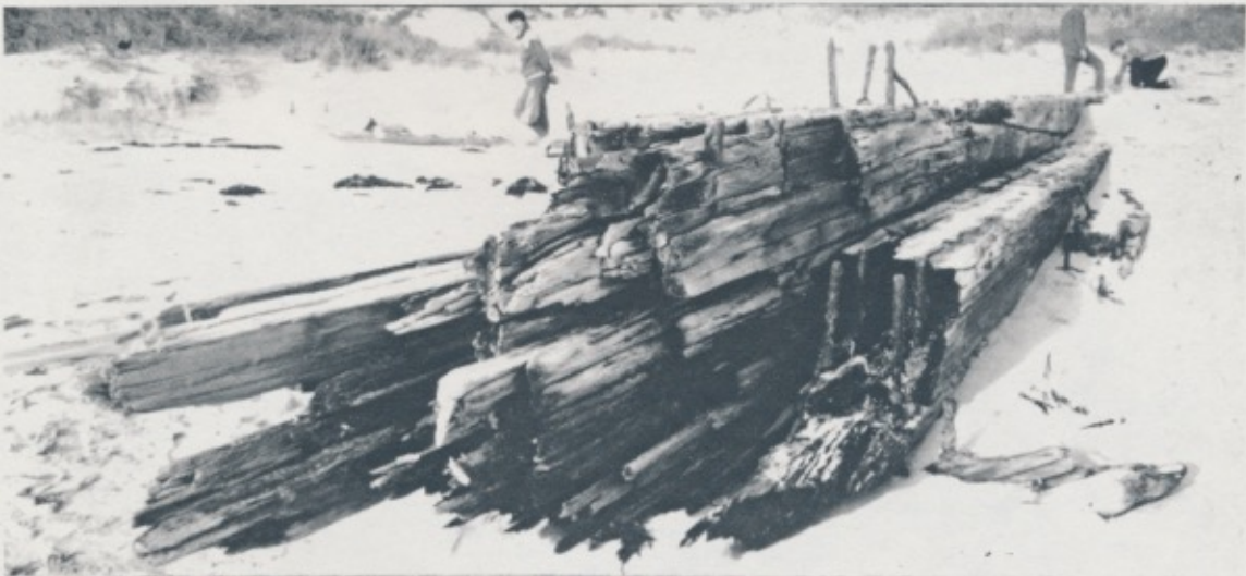
The sea end of the keel timbers - damaged by fire at some time in the past - Photograph by Brad Sergeant
