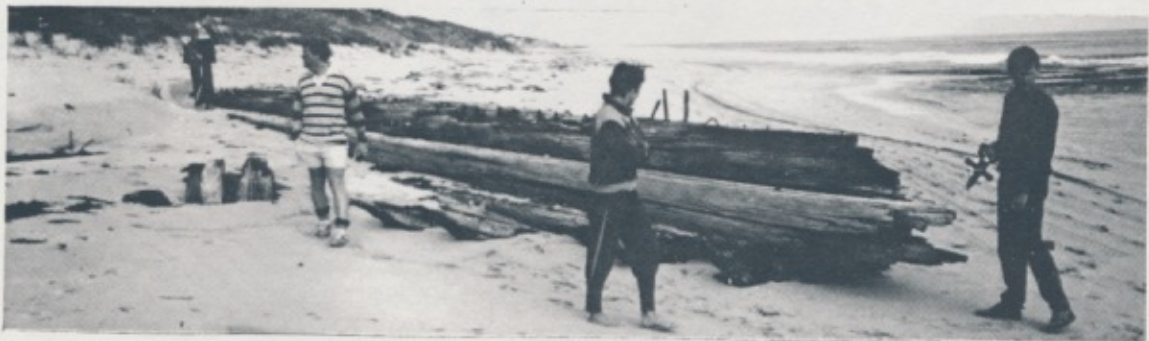
The sea end of the keel timbers - damaged by fire at some time in the past - Photograph by Brad Sergeant
