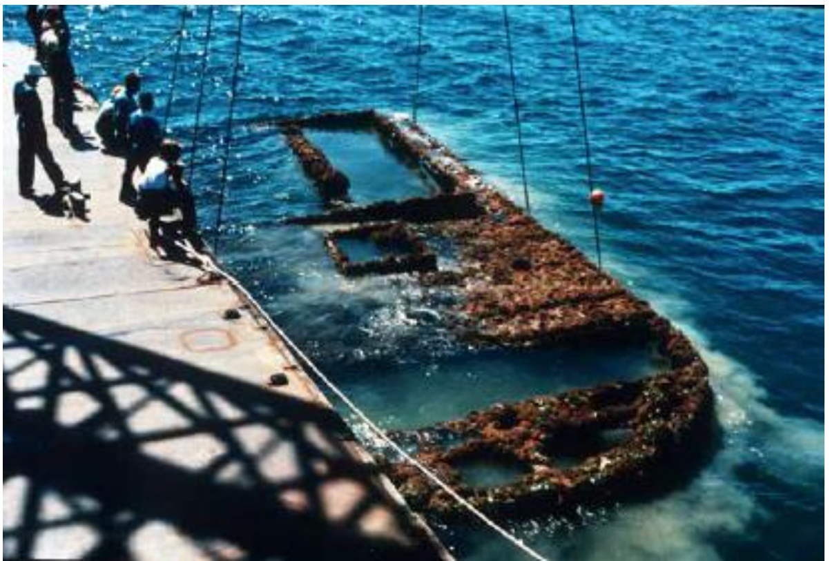
Figure 23 The North Mole Barge raised by the Pelican and moving to new site (West Australian Museum).
